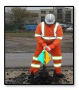
iv) Reposition your feet shoulder-width apart, and using slow, smooth movement, move the lever to the other side of the switch stand.
